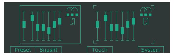
The front page shows the process settings for both channels, allowing you to see the complete setup without flipping between the channels using the CHAN1 and CHAN2 buttons.
