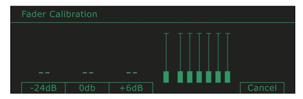
Fader calibration is necessary only after a firmware upgrade or after a faulty fader is replaced. The procedure is as follows:
