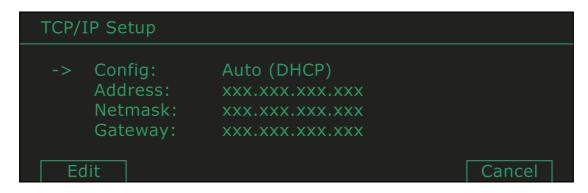
The network interface may be configured automatically if your network has a DHCP server, or manually. Toggle between these states by pressing EDIT when the Config menu item is indicated.
