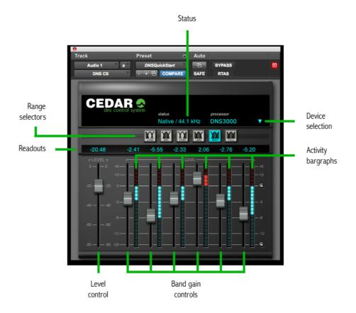
You must always remember that the Control System is precisely what it claims to be: a Control System. It performs no audio processing. To process an audio stream you must route it via the DNS3000 itself using the AES/EBU or SPDIF I/O. You can do this, for example, by using an insert point within the Pro Tools mixer.
