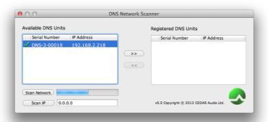
The Network Scanner must be run in order to allocate which DNS3000 units on an Ethernet network are available to a given instance of the DNS CS. Until it is run, the DNS CS will only be able to see DNS2000 units connected by USB. Allocating a unit to one PC/Mac does not prevent it being allocated to another, but is not recommended.
