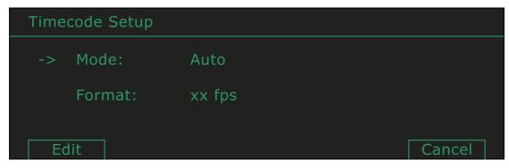
This page allows you to select automatic or manual selection of the timecode format. Toggle between the two states using the spinwheel when Mode is selected.
