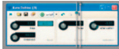
Auto Dehiss in M-S Mode, attenuating hiss in just the stereo signal.
