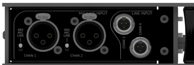
If required, connect the outputs from line-level analogue sources to the balanced TA3 mini-XLR inputs of channels 3 & 4.
