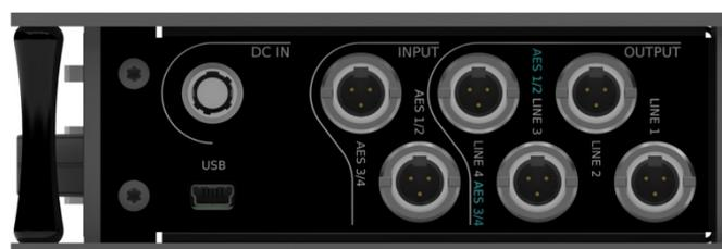
Connect the DNS 4's AES3 or analogue outputs to the corresponding input sockets of your receiving devices. The analogue or digital output selection is made using **channel button 3** in the Setup page.
