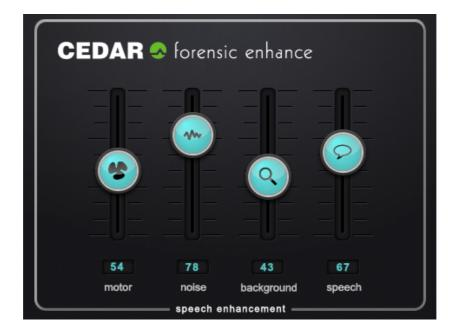
There are four processes, each with a single control. The controls have scales from zero to 100. There are no units for these numbers.
